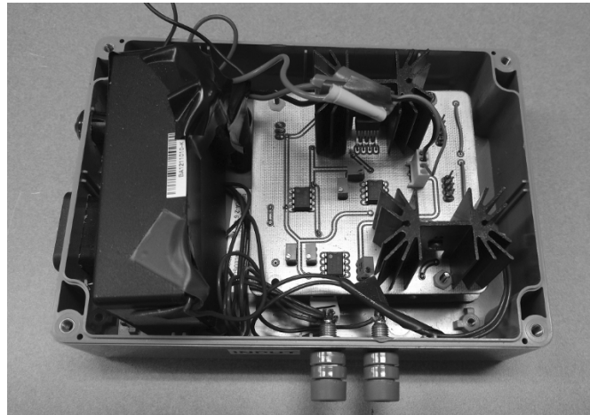
Figure 6.5. A photograph of the custom electronic circuit for detecting the response of the force sensing suture anchor.
